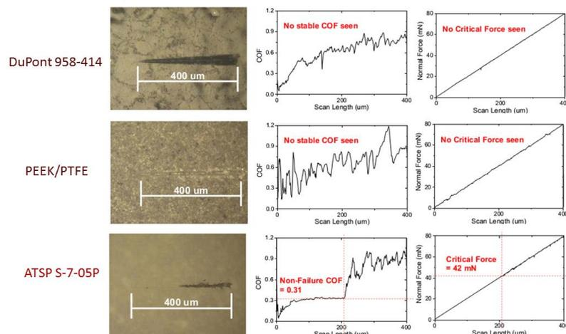
**Fig. 4:** Results of scratch experiments conducted on PTFE-, PEEK-, and ATSP-coated cast-iron disks.
