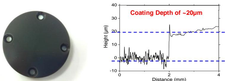
**Fig. 2.** (Left) A representative spray coated disk. (Right) Profilometry scan indicating coating thickness (which is consistent at 20-40 ± 5 microns)
