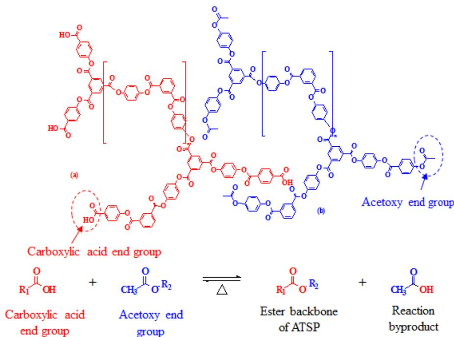
**Fig. 1.** Chemical structure of ATSP resin
