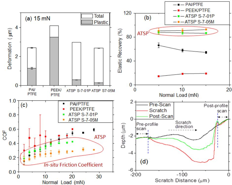
**Fig. 3:** Elastic versus plastic deformation for PTFE-, PEEK-, and ATSP-coated cast-iron disks.
