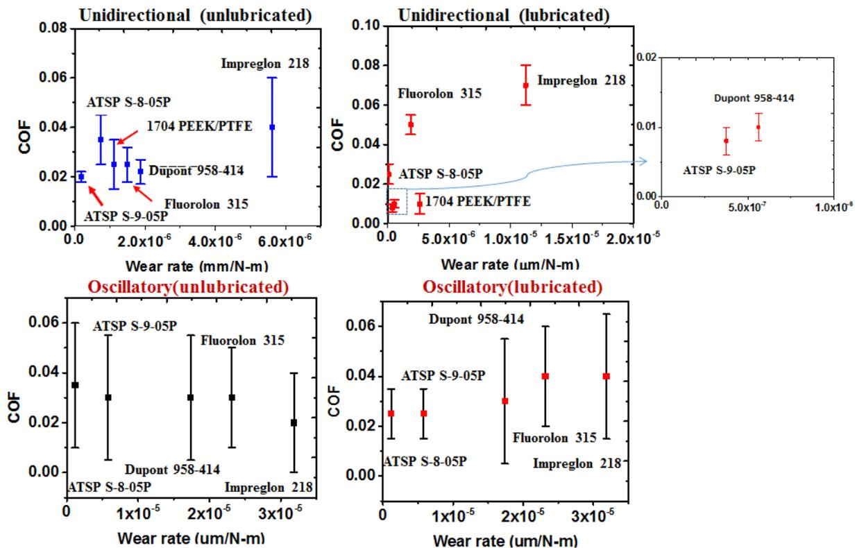
**Fig. 5.** Friction coefficient (x-axis) vs. wear rate (y-axis) of ATSP versus several commercial polymeric
